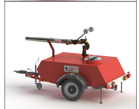
1000L Trailer with HM80 and LTC1800 Self Inducing Cannon
